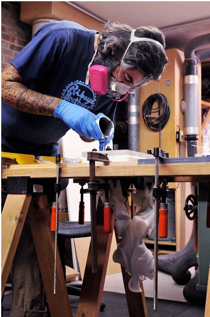
Studio assistant Gary Mellon fills the hollow, plastic model with resin. COURTESY BARRY X BALL STUDIO.
